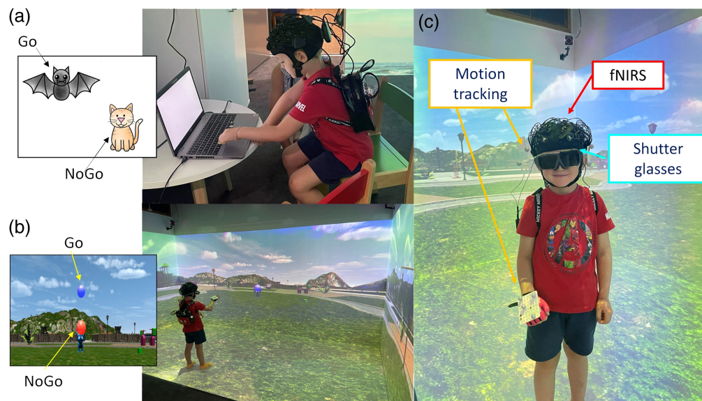
Fig. 1 Experimental protocol. Children performed a computerized version of the go/no-go task sitting in front of a computer (a) and a VR version while freely moving in a VR CAVE (b). In the CAVE, children wore the fNIRS cap in conjunction with motion tracking markers and custom-made shutter glasses.
