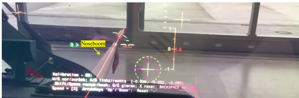
Fig. 10 Manual calibration of the full internal tracking in order to align it with the real world using the noseboom as a reference. This is then used as a reference to calibrate the external tracker with it.
