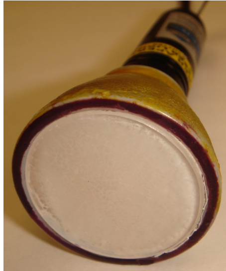
Fig. 3 A lamp style LD-pumped phosphor-converted white light source.
