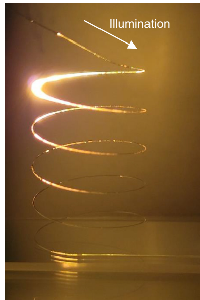
Fig. 13 Printing a small spiral structure built using DFG and a 125 \mu\text{m} diameter optical fiber.
