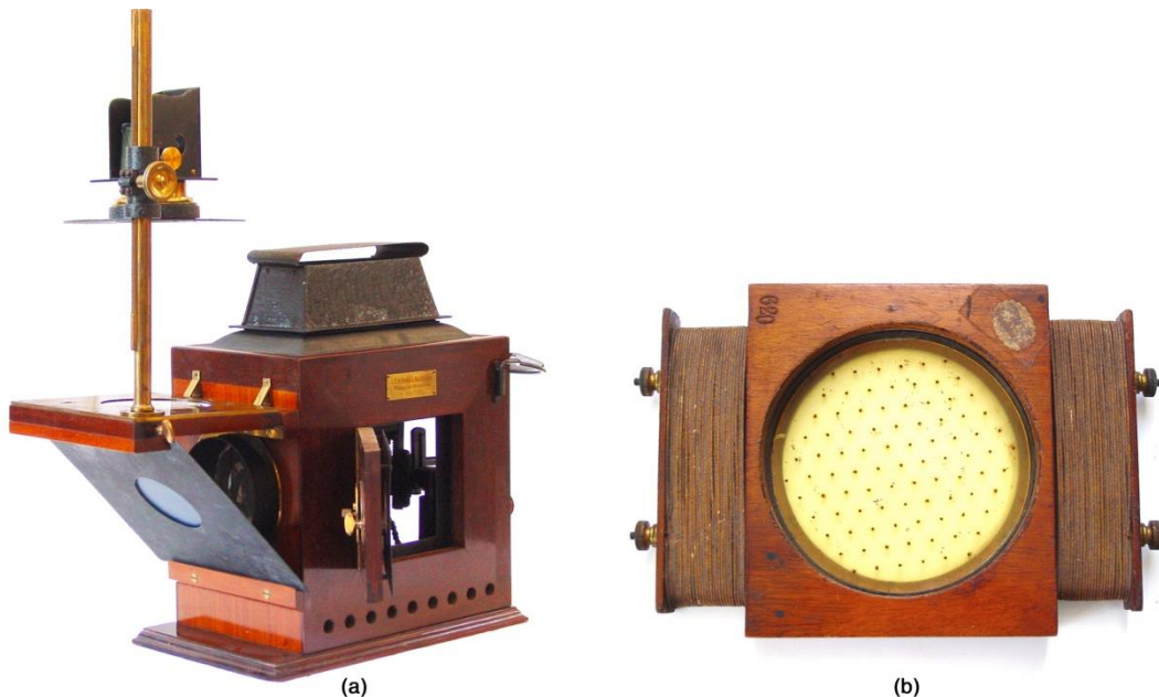
Figure 4. (a) The projection apparatus prepared for experiments performed horizontally. (b) Ewing's apparatus, where tiny magnetic needles (now missing) on an array of pins materialize magnetic field lines.
