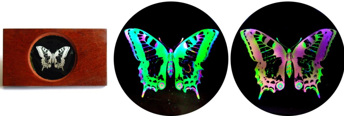
Figure 14. Gypsum preparation for projection in polarized light. Complementary colours as shown by the 90° rotation of the nicol.
