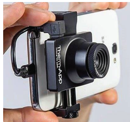
Fig. 61 Thermal imaging as a smartphone application.
