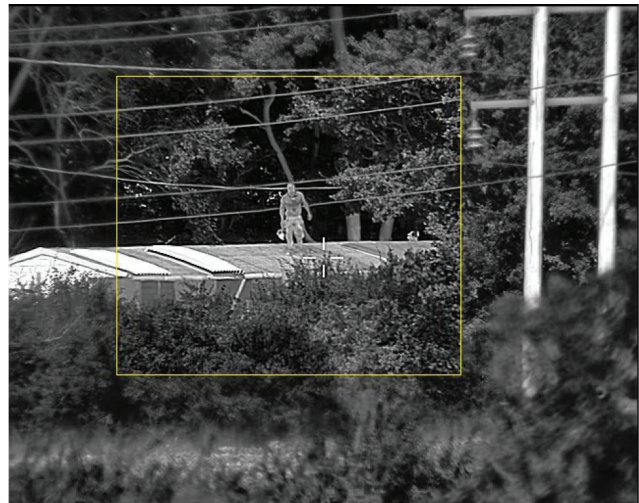
Fig. 60 Example of atmospheric turbulence mitigation applied in central boxed region.
