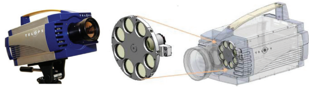
Fig. 58 LW camera with filter wheel system
