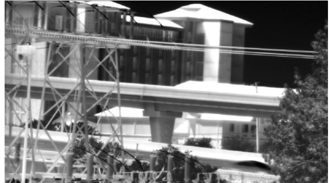
Fig. 28 LWIR image taken with a 720 \times 1280 FPA having 5 \mu\text{m} pixels. An f/1 lens was used.
