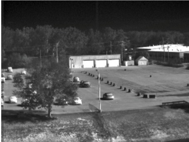
Fig. 18 30 mK infrared imagery from an MWIR PbSe FPA at 230 K and 400 frames per second.
