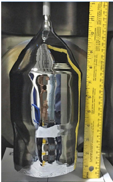
Fig. 14 GaSb boule capable of yielding over 70 6-inch wafers.
