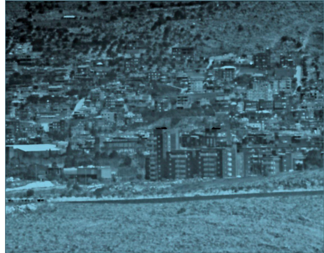
Fig. 6 Image registered with a demonstration camera containing the 15 \mu\text{m} pitch, 640 \times 512 \text{ LW FPA} , operating with F/2.7 optics at 77 \text{ K} and a scene distance of about 5 \text{ km} .
