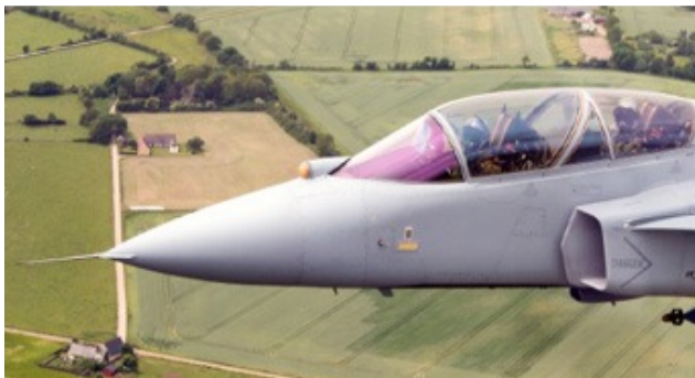
Fig. 39 Embedded version of the IRST during flight trials.
