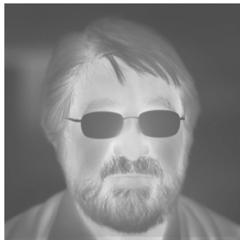
Fig. 15 Image from a QWIP FPA at V \sim -1.1 V bias and T = 61 K.
