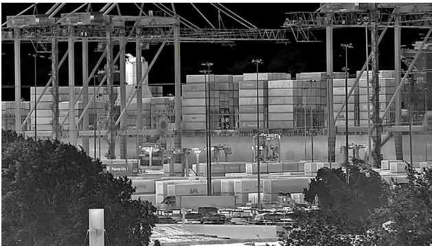
Fig. 28 Image of a container ship at ~ 1.6 km being unloaded taken by an MWIR HgCdTe array with 75 mm f/2.8 optics.
