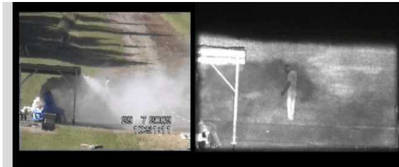
source: ISL, 1.5µm laser gated viewing, recognition of person through smoke
