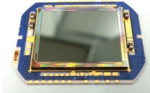
Fig. 11 Photo of a new Type II superlattice FPA with a resolution of 1280 × 1024 and having 12 μm pitch pixels.
