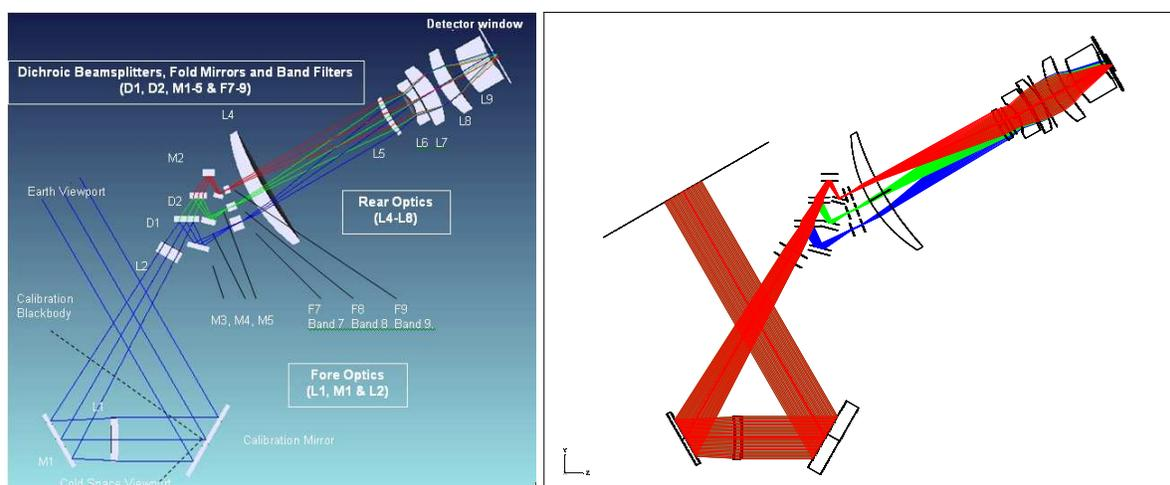
**Fig. 2.** TIR optical layout. The rear optics are defined downstream of F7, F8, F9.
