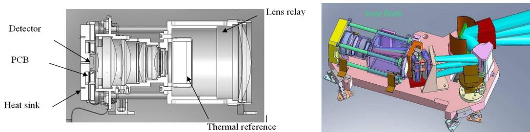
**Fig. 4.** TIR rear optics structural design – Invar rods maintain the system athermalisation.
