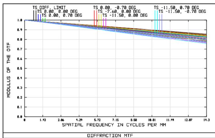
Fig. 7. MTF at 3 field points for Band 9, nominal design result
