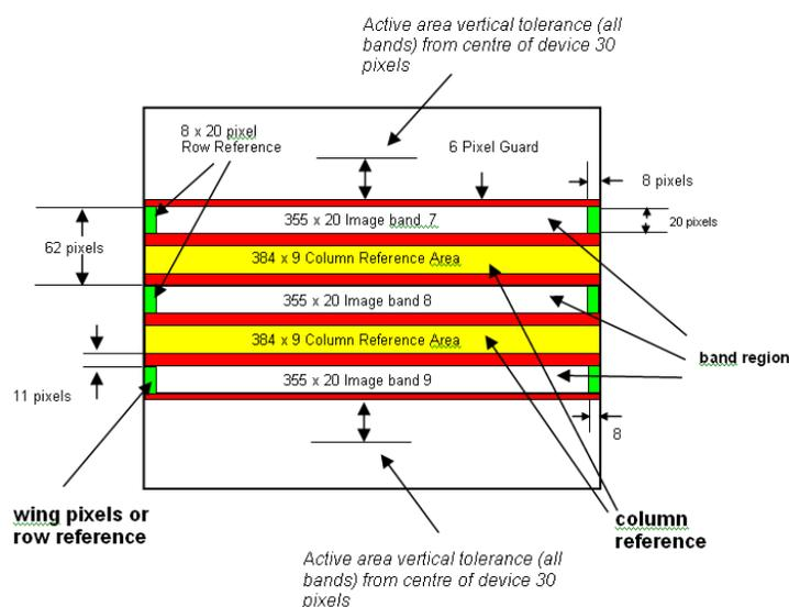
Fig. 6. Sketch of Operating bands for the TIR detector
