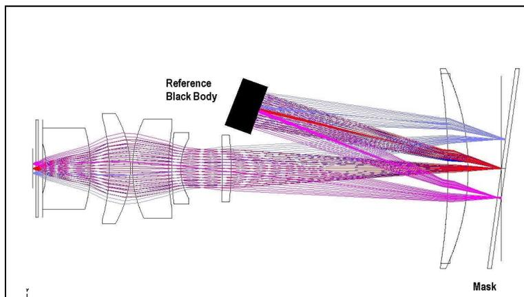
Fig. 5. TIR rear optics showing the internal thermal reference blackbody
