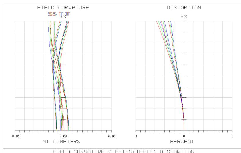
**Fig. 8.** Field Curvature and Distortion results from the TIR design
