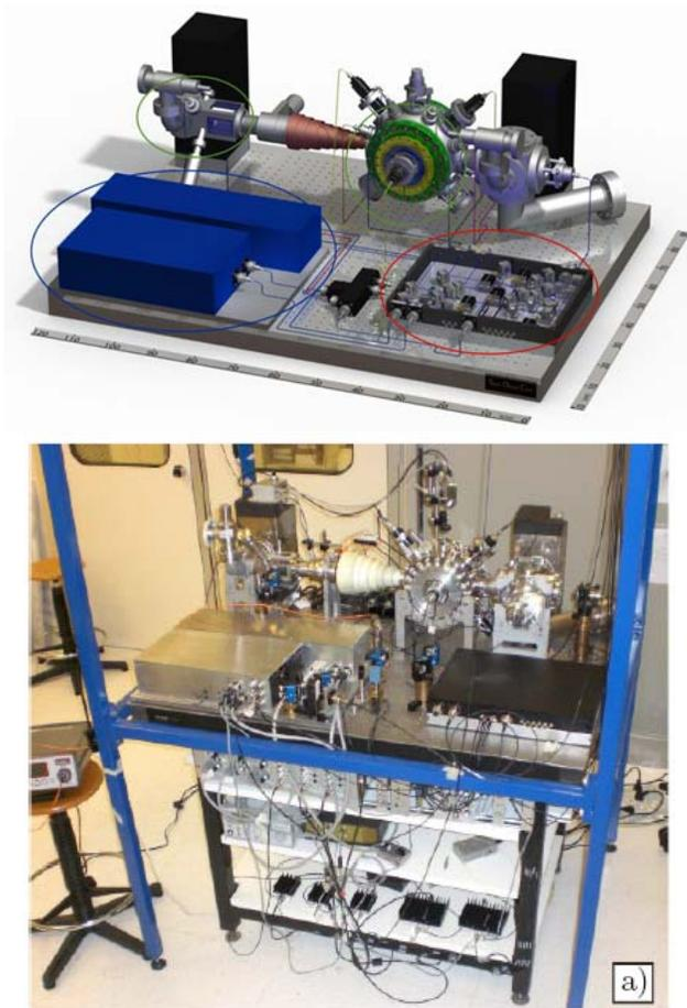
**Figure 4.** Top: design of the breadboard (120 cm  $\times$  90 cm) for cold Sr production and trapping (LENS/Università di Firenze). The blue boxes contain the 461 nm laser, the red-circled box is the frequency generation system. The two black columns are ion pumps. The atom source is circled green (top left), the frequency generation subsystem red.
