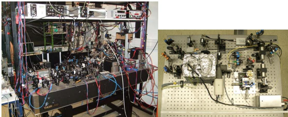
**Figure 5.** Left: optical table with the vacuum chamber and cooling/lattice lasers. Right: clock laser system. At bottom right is the 1156 nm diode laser. Silvery box contains the ULE cavity (Universität Düsseldorf).
