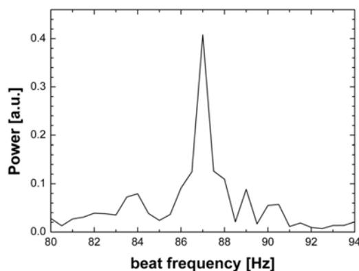
**Figure 3.** Beat spectrum between two independent clock lasers, one for Sr (698 nm), the other for Yb (578 nm), after transport of the Sr clock laser from Braunschweig to Düsseldorf, showing a combined linewidth at the 1 Hz level. Measurement time: 2 s; 0.5 Hz resolution.
