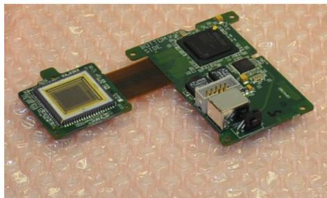
**Fig 10** LCMS camera and processor
