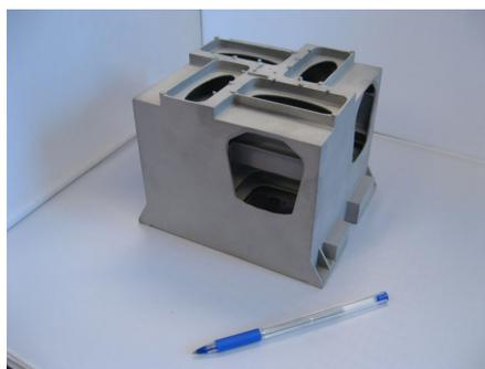
**Fig 5** Cast aluminium housing
