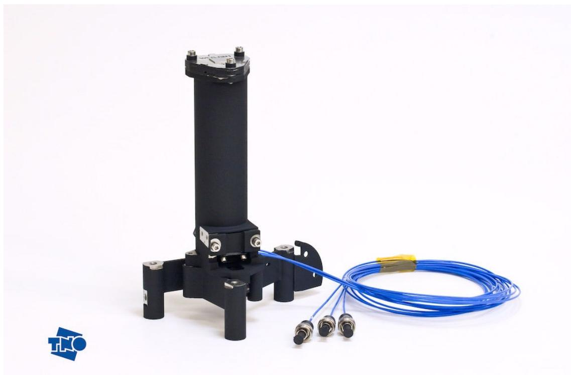
**Fig. 5** The WFS qualification model. The WFS's exterior is black for stray light reasons. The interface to the SiC GAIA-focal plane is by 3 tangential invar flexures. Three calibration fibres can be seen (blue). The WFS is 150 mm high, and weighs less than 500 grams.
