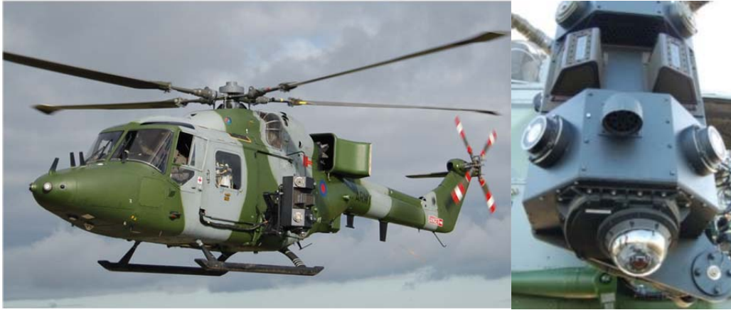
Figure 6 - Miysis DIRCM during CDAS Flight Testing in 2012
