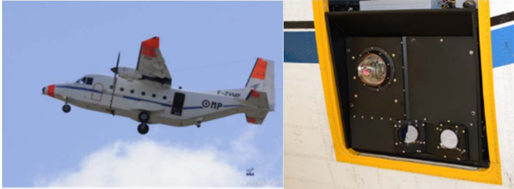
Figure 7 – The Miysis DIRCM System during the 2014 Flight Trials (Photo's courtesy DGA)
