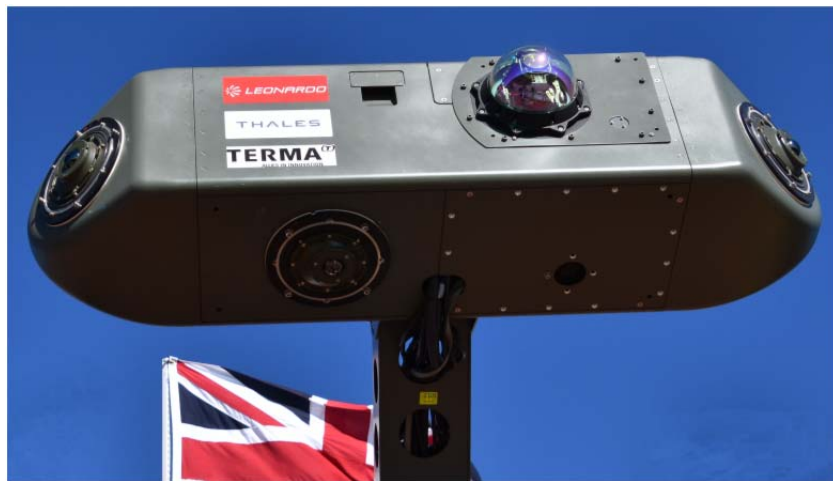
Figure 11 – The UK DIRCM System (including Miysis) at the Recent Missile Live-Fire Trial
