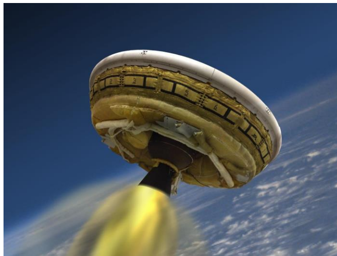
Figure 6. An artist's rendering of the LSD fully deployed in the powered flight phase 9 .
