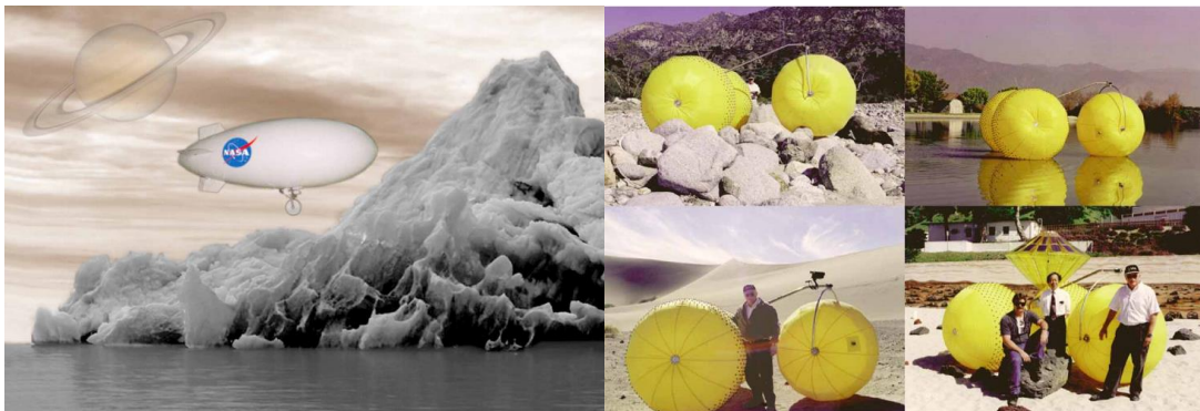
Figure 12. (Left) Titan Aerover blimp with inflatable wheels and (Right) inflatable rover concept vehicles 13 .
