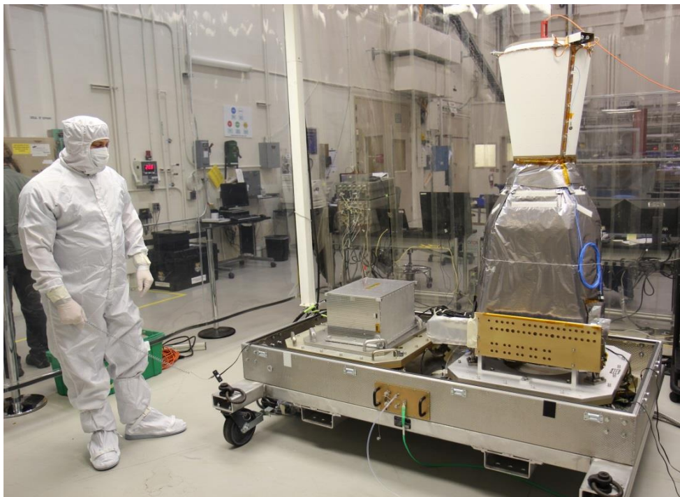
Figure 3: Photo of the GLM Electronics Unit (left) and Sensor Unit (right)
