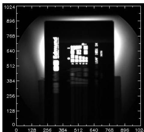
Fig. 3 : Picture of the USAF target (light intensity multiplied by 5 to show ghost and smearing)
