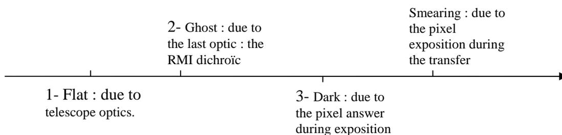
Fig 4 : Order of apparition of the defects in the image creation process
