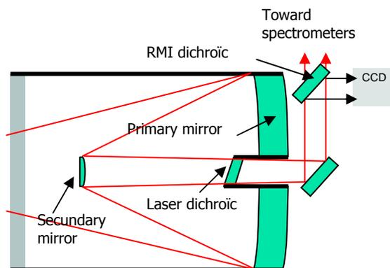
Fig 2 : light path in the telescope
