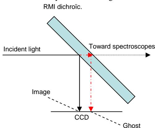
Fig. 5 : light rays on the RMI dichroic
