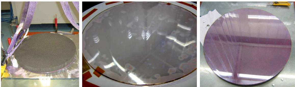
**Fig. 3.** (left) Foamglas® boards assembled to form the panel core. (center) Hot slumped glass shell in contact with its forming mandrel. Only a narrow corona along the glass circumference deviates from the mould shape. (right) Mirror panel after the curing of the glue and the vacuum release.
