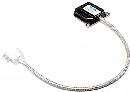
Fig. 2. A fiber coupled laser light module for automotive front lighting applications, which is composed of a high power 450nm wavelength blue laser module, a transporting multi-mode optical fiber and a remote reflective laser phosphor packaged in a metal head.
