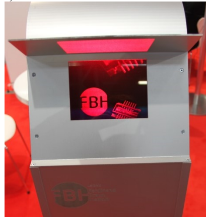
Fig. 6. Picture of a hologram demonstrator using a 633 nm DBR-TPL for illumination.
