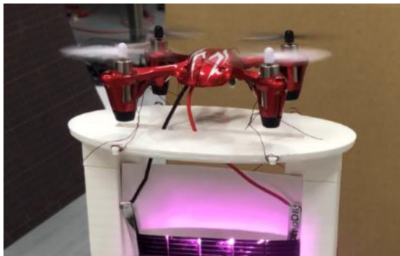
Fig. 3. Dynamic charging to toy-micro drone using VCSEL. Limited to a few cm floating due to fixed beam system.
