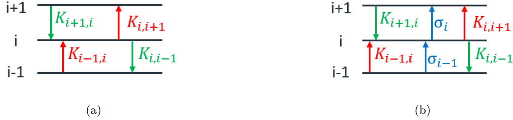
Figure 1: Example 3-level systems showing the populating and de-populating processes for an ionization level i both (a) without photo-ionization and (b) with photo-ionization.
