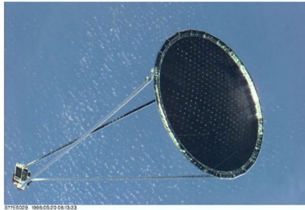
Figure 1. Mylar space project (Inflatable Antenna Experiment, IAE). This test consisted of deploying and maintaining of 14 m parabolic aperture antenna in the space environment. Since the vacuum environment, 3e^{-4} psi is good enough to keep the surface tension. [8]
