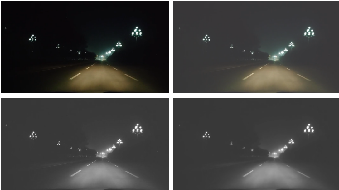
Figure 2. The upper left corner is the original image, the upper right corner is the image after contrast stretching, the lower left corner is the image after grayscale processing, and the lower right corner is the image after median filtering and bilateral filtering
