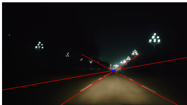
Figure 6. Draw the filtered directly on the original image and mark the intersection points
