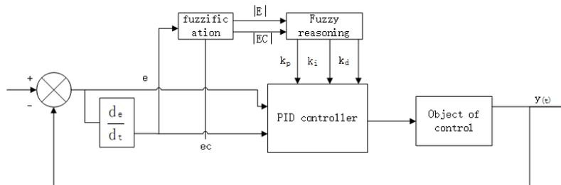
Figure 1. Principle diagram of fuzzy controller.
