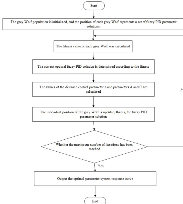
Fig 4. GWO-Fuzzy PID algorithm flowchar.
