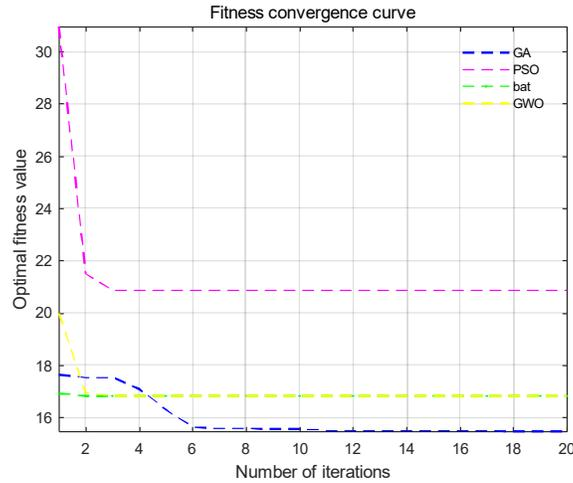
Figure 7. Comparison of convergence curves for four algorithms.
