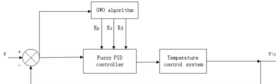
Figure 2. Optimization of fuzzy controller parameters based on GWO.
