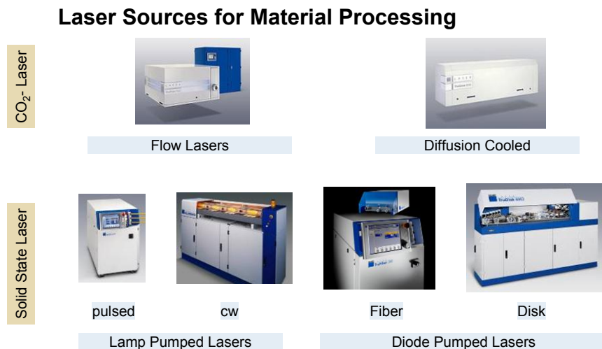
Figure 1: Laser beam sources for material processing in use today. This overview excludes excimer lasers – they are used in micromachining and photolithography applications. Diffusion cooled and fast flow CO 2 lasers dominate the market for sheet metal cutting. Most solid state lasers for material processing are fiber delivered, such as thin disk and fiber lasers. This paper will focus on the diffusion cooled CO 2 laser with coaxial discharge and helix resonator, the diode-pumped solid-state thin disk laser as well as the high power diode lasers used to pump solid-state lasers.
