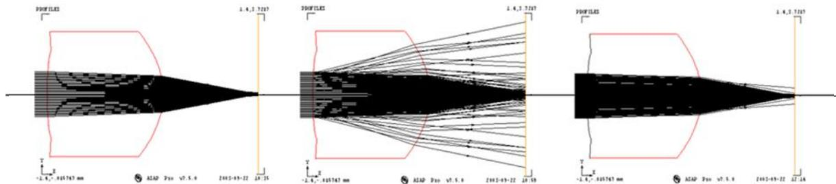
Figure 2: simulation of lens performance with ideal profile, large draft angle, optimized draft angle
