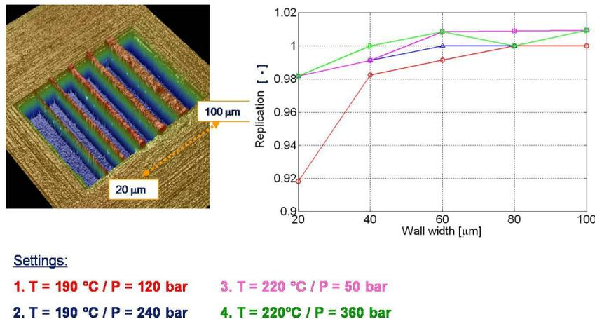
Figure 9: Combined influence of mold temperature and pressure on the replication of microstructures via hot-embossing
