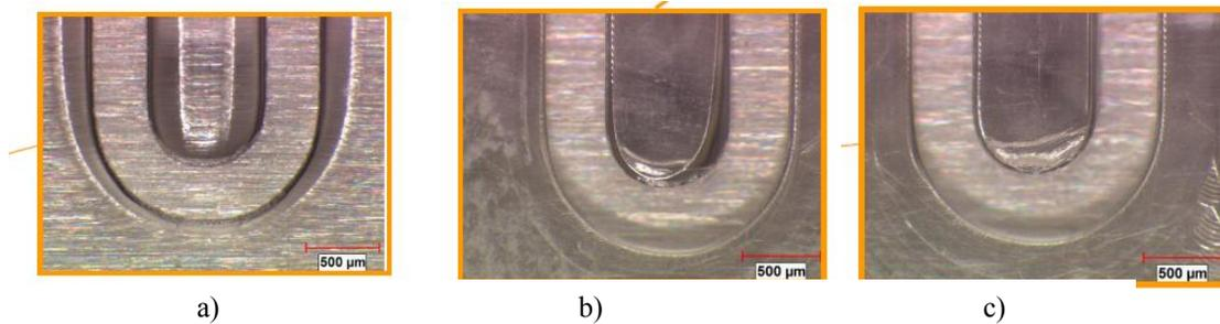
Figure 8: replication of a section of a serpentine-like microfluidic channel via hot-embossing at different mold temperatures: a) 140 °C, b) 190 °C, c) 220 °C
