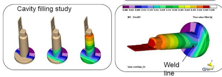
Figure 5: Numerical flow analysis of an injection molded part using Cadmould<sup>2</sup> showing location of the flow front in time
