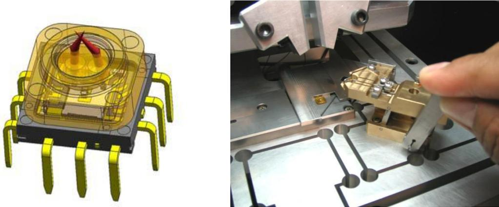
Figure 11: Philips Twin – Eye Laser Sensor – product and tester
