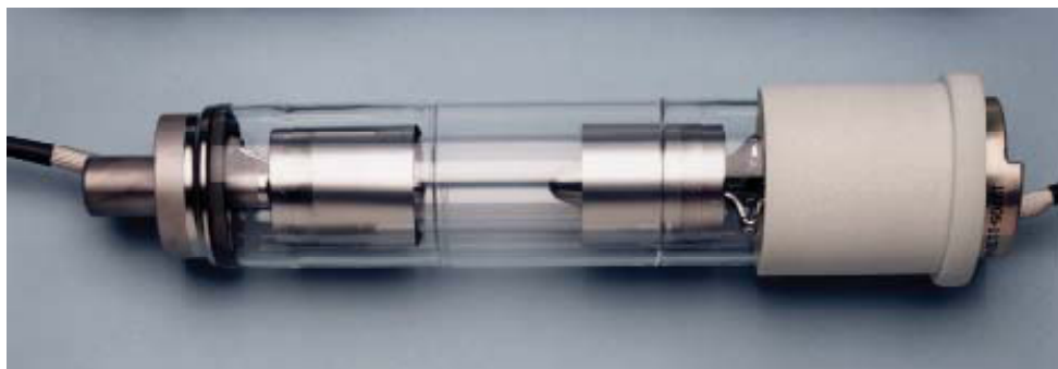
Figure 3. AN/ALQ-157 IRCM System Cs Arc Lamp [5]
