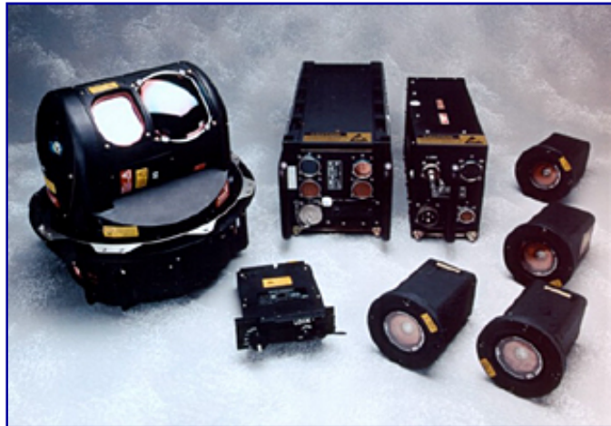
Figure 7. Early Lamp-based DIRCM System (also known as FIRCM) [9]
