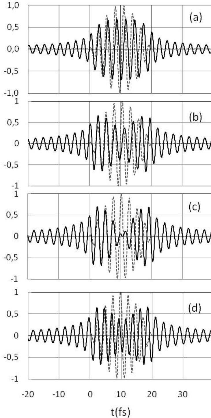
Fig.3. Normalized temporal envelopes of fs pulse (11) ( $t_0=20\text{fs}$ ), propagating in a free space (dotted lines) and tunneling through the gradient barrier (solid lines),  $\Omega = 2.45 \cdot 10^{15} \text{ rad/s}$ ; carrier frequencies  $\omega_0$  and detunings  $\Delta$  at figures 3a – 3d are
