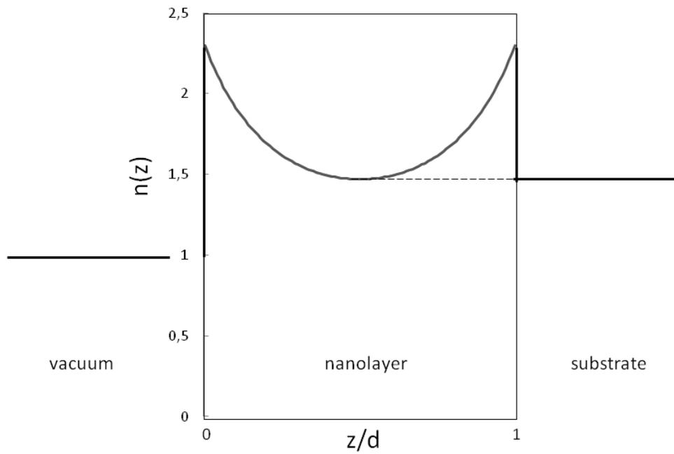
Fig.1. Normalized profile of dielectric susceptibility  $U^2(1)$  inside the gradient photonic barrier, providing the tunneling of EM wave through barrier with thickness  $d$ , located on the substrate;  $z/d$  is the normalized coordinate across the barrier.
