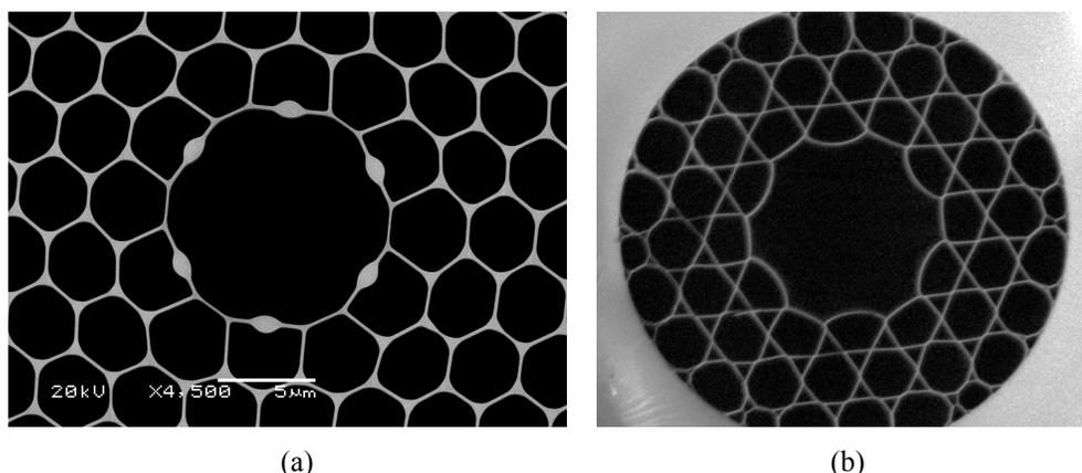
Figure 4 Scanning electron micrograph of (a) a HC-PCF with anti-resonant core wall features and (b) a hollow core PCF with a large pitch few ring cladding.
