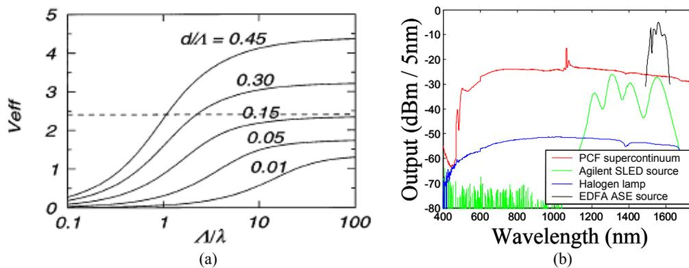
Figure 2 (a) Variation of  $V_{\text{eff}}$  with  $\Lambda/\lambda$  for various relative hole diameters  $d/\Lambda$ . The dashed line marks  $V_{\text{eff}} = 2.405$ , the cutoff V value for a step-index fiber<sup>[3]</sup>. (b) A plot of the output spectra of different light sources to compare the broadband supercontinuum generated in PCF against the low power or narrow bandwidth alternatives.
