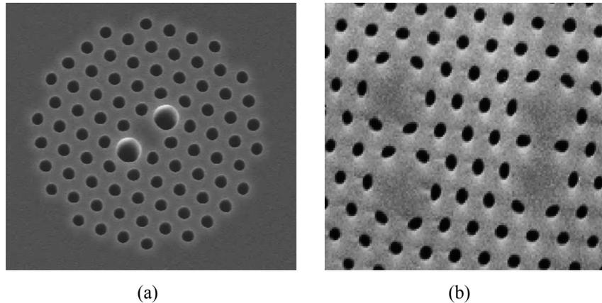
Figure 3 Scanning electron micrographs of (a) A highly birefringent photonic crystal fiber with two holes with a larger diameter placed symmetrically about the core and (b) an example of a photonic crystal fiber with multiple cores, here there are two pairs of cores the strongly couple to each other.
