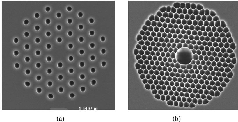
Figure 1 Scanning electron micrographs of (a) Photonic crystal fiber that confines light to a high index silica core via total internal reflection and (b) a hollow core photonic crystal fiber that guides light in a low index air core using photonic band gap confinement.
