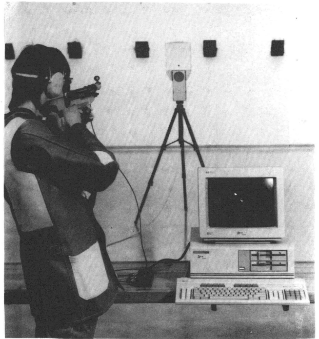
Figure 4. Laser training equipment for marksmen. The transmitter emits a continuous light beam during sighting and shooting and enables recording of the sighting trajectory and triggering event. The system can be attached to, and easily calibrated for various weapons (by courtesy of Noptel Ky).
