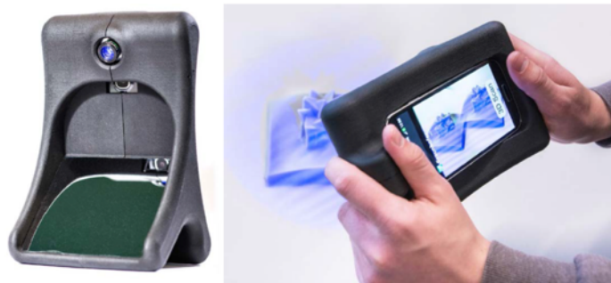
Figure 4. Design prototype of the Fraunhofer IOF low-cost 3d capturing development-kit. (source: Fraunhofer IOF)
