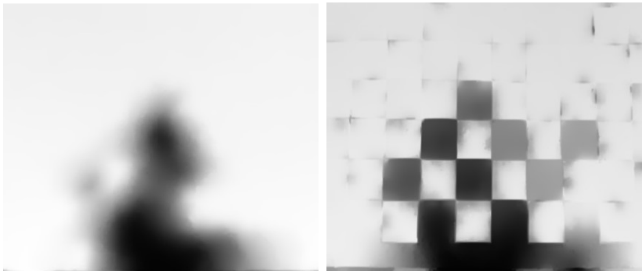
Figure 4. Measurement problems in the lower and central image parts for distances near the minimum working distance: White paper at 150 mm (left) and the object checkerboard at 160 mm (right).
