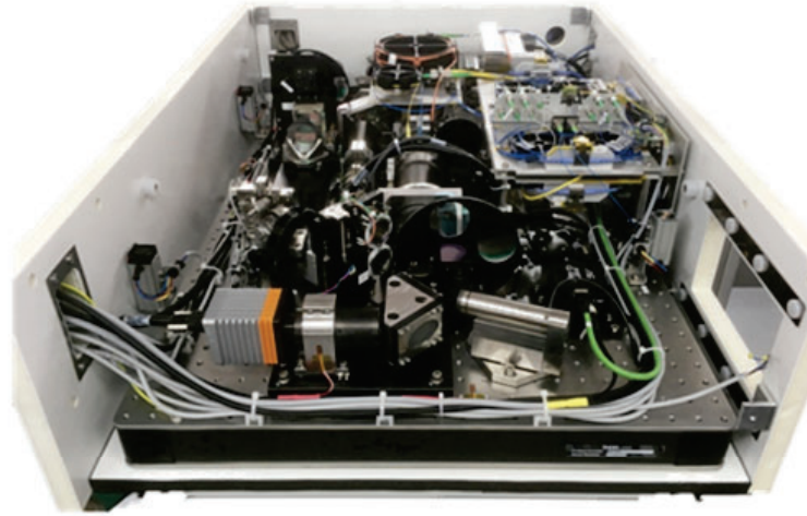
Figure 3. CARO instrument optical bench before box closure.
