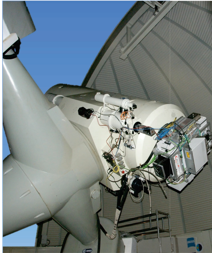
Figure 4. CARO instrument mounted to ESA OGS telescope.
