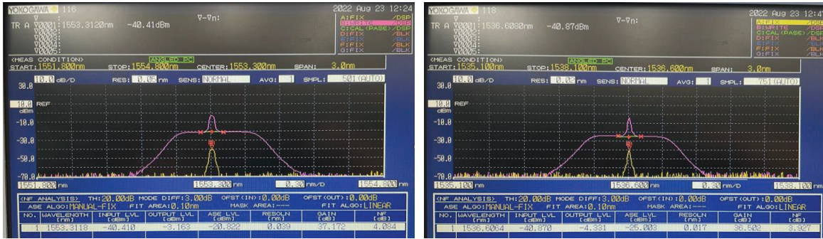
Figure 8. Typical optical spectrum analyzer LNA Noise Figure measurement display near 1550nm (left) and 1535nm (right) for input level of -40 dBm, span = 3 nm. Input signal is yellow trace, output signal is magenta trace. Note that NF measurement includes optical test cable losses of ~0.35 dB.
