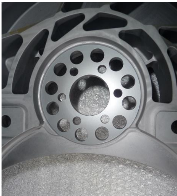
Fig. 4. Detailed view of P1 SiC panel ready for assembly Fig. 5. CMM check of the main structure assembly
