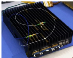
Fig. 1 Laser Transmitter showing interface and cooling fins on the base.
