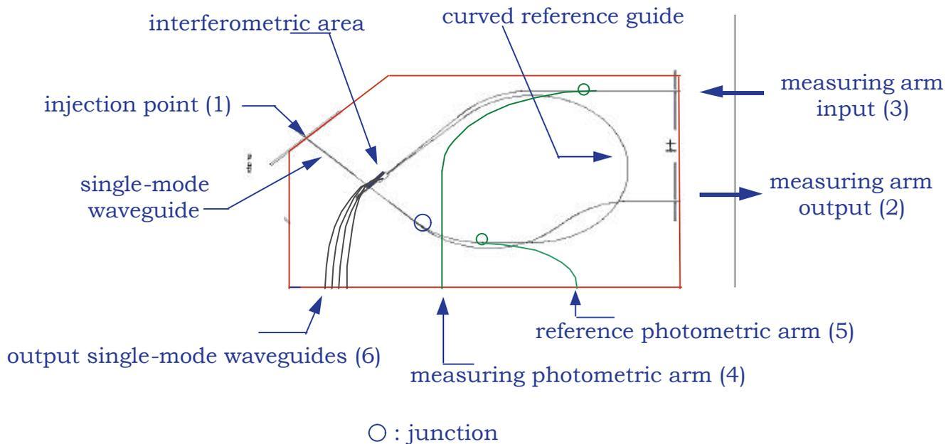
**Fig.4** : Scheme of the optical circuit
