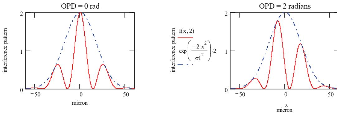
Fig.3 : Fringes moving with the object displacement
