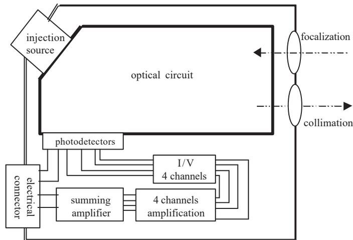
**Fig.5** : scheme of a measuring head
