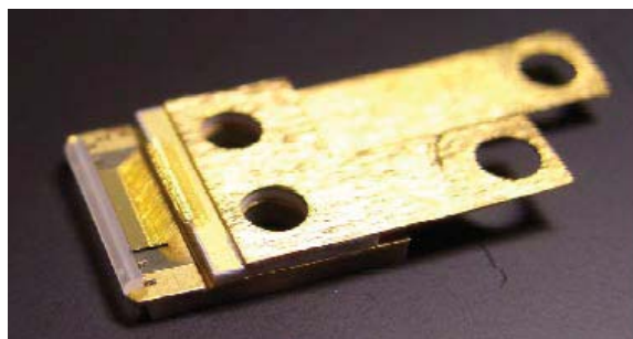
Fig. 5. Preliminary design of QCW high power laser bench
