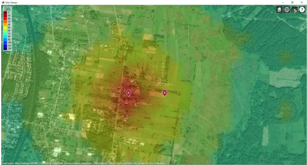
Figure 6. The electromagnetic field strength when operating at 292 MHz frequency
