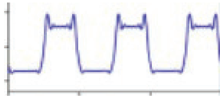
Figure 3: 2D trace of the batwing effect when measuring a periodic grating.
