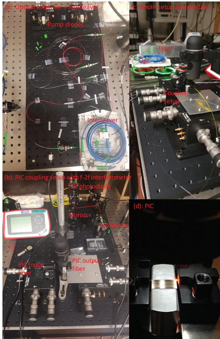
Figure 4-1 :Pictures of the photonics oscillator setup: (a) Optical amplifier + interleave,(b) PIC coupling setup with f-2f interferometer,(c) whole setup and (d) zoom onto the PIC in action
