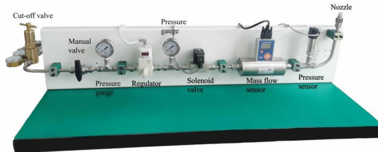
Figure3. Hydrogen jet equipment
