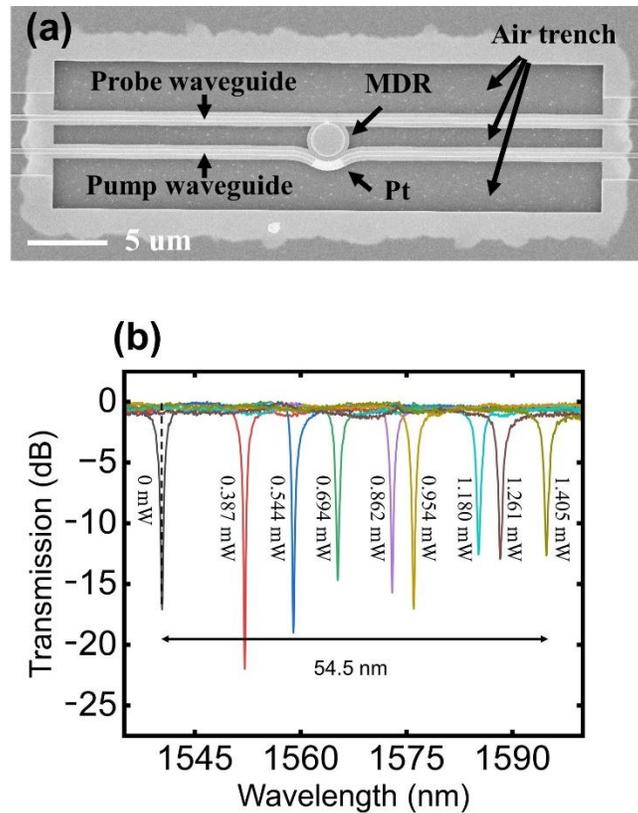
Figure 2. (a) Top-view SEM image of the fabricated device. (b) Measured transmission spectra of the all-optically tunable filter with different pump powers. The ER is shown by the dashed line at the first resonant peak.
