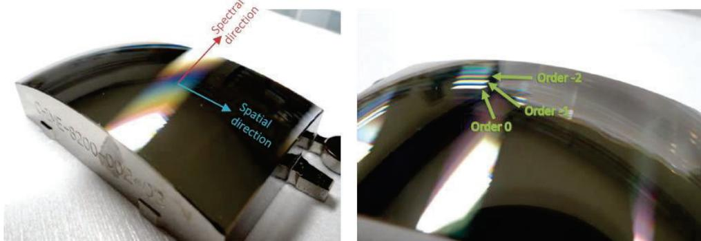
Figure 8: Pictures of an actual dual-blazed UPM-shaped grating. The grooves are parallel to the workpiece long edge, (spatial direction), while the spectral dispersion direction is orthogonal to it. Order identification is proposed on the right panel.
