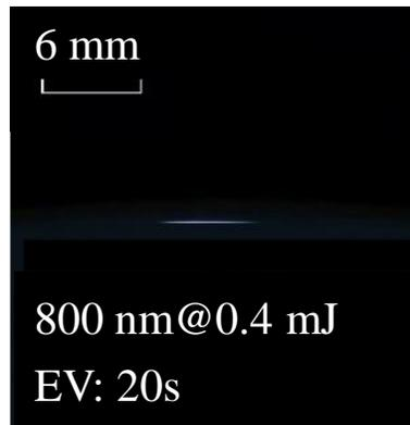
Figure 1. Filamentation of 800 nm femtosecond laser in air (laser energy: 400mJ, EVs: 20s)
