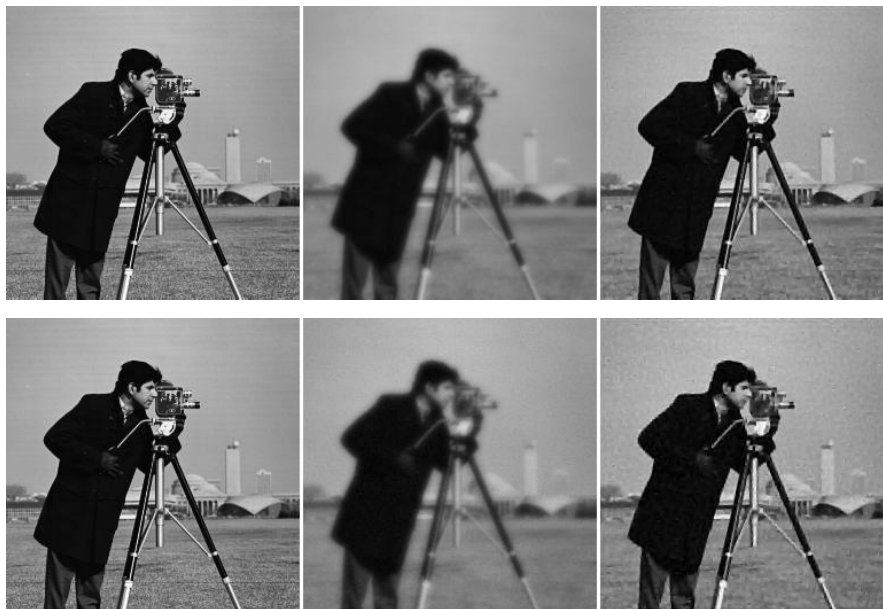
Figure 4. Deblurring results with the PCD-SESOP0 algorithm: Original image (left), measured blurry and noisy image (middle), and restored (right). Top images refer to the experiment with \sigma^2 = 2 , and the bottom ones for \sigma^2 = 8 .
