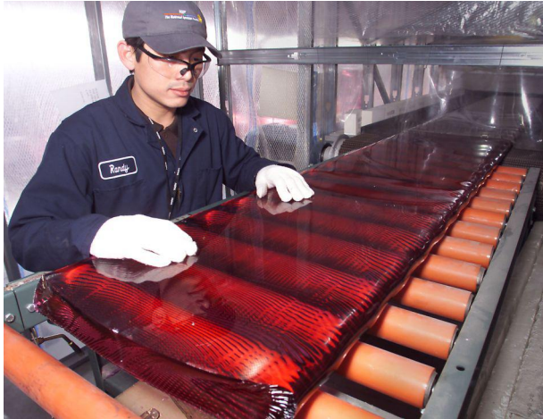
Figure 4 left: NIF laser glass emerging from a continuous glass melter. Right: NIF wedge focus lens.
