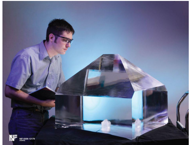
Figure 5 left: KDP crystal grown with mid-1990s technology. Right: NIF KDP crystal grown via rapid-growth technique.
