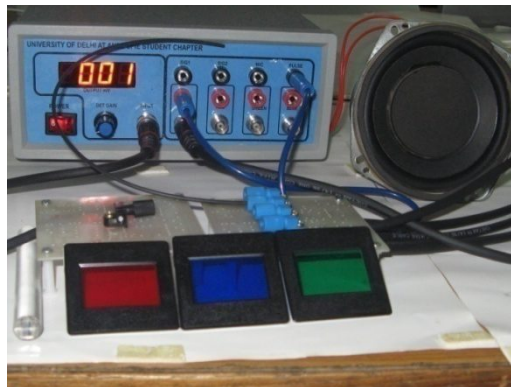
Fig. 3(e): Set up for demonstrating WDM
