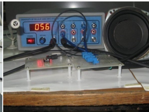
Fig. 3(d): Demonstrating Optical Communication (Analog, Digital and Voice)
