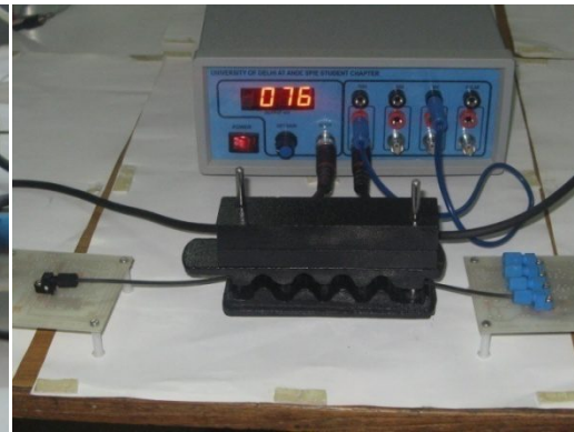
Fig. 3(b): Determine bending losses in a fiber
