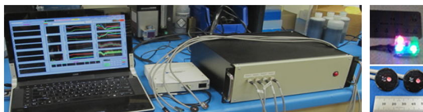
Fig. 2 The benchtop PPG sensor (on left) including the laptop, data acquisition card, and sensor interface electronics (from left to right). The right panel shows the visible (upper) and NIR LEDs (lower) used in this study.
