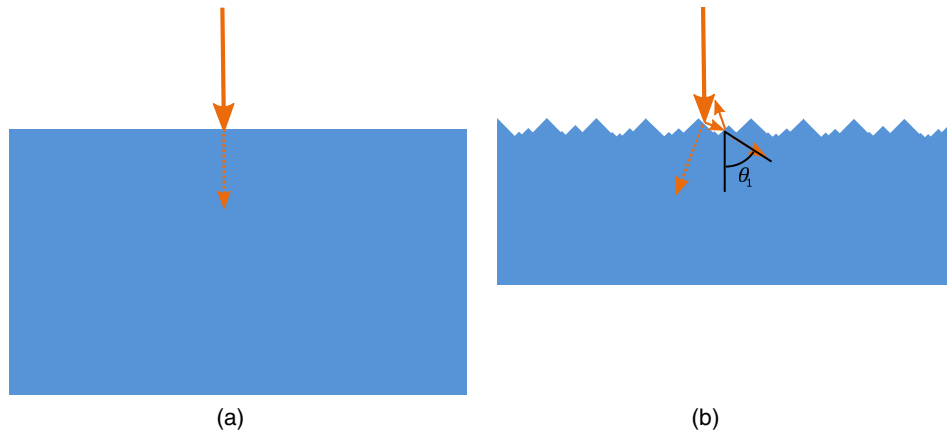
Fig. 7 (a) The single pass LPEF enlarged planar substrate that would generated the same absorption results like the (b) structured substrate.
