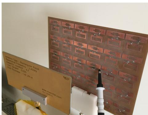
Fig. 6 Voltage signal measurement via digital oscilloscope probe.
