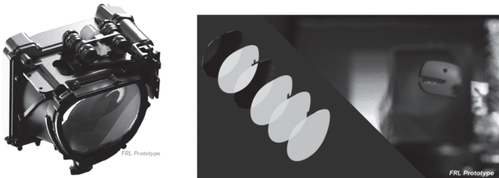
Figure 18.7 Facebook Reality Labs VR varifocal lens based on stacked LC lenses, and operation example.
