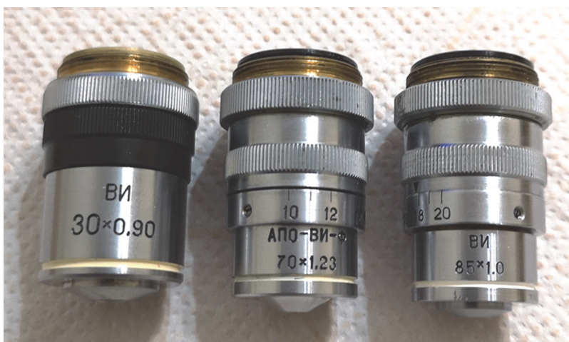
Figure 1.25 Photographs of some Russian mass-produced objectives for water immersion.
